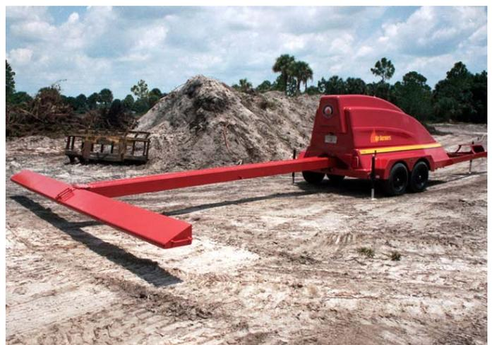
Figure 6—Trench burner.
