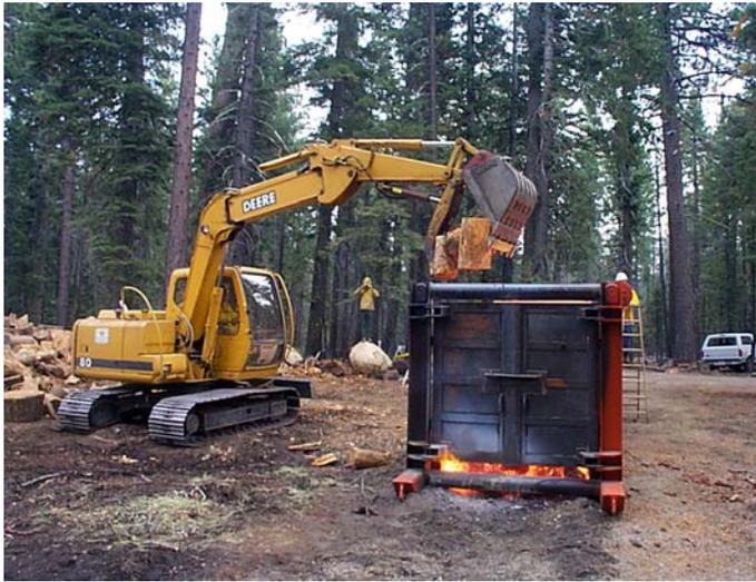
Figure 4—Loading fuel into ACD (full operation).
