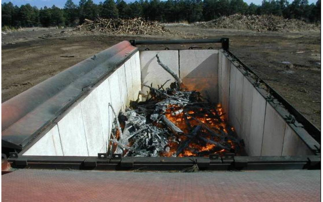
to local sawmills, and firewood is donated to the public. The branches, also known as slash, are either turned into mulch or burned into ash. Burning timber in the open creates excessive air pollution, so the Lab purchased three Air Curtain Destructor (ACD) units to significantly reduce air emissions.
