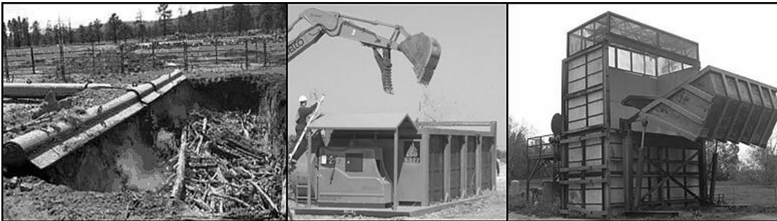
Figure 2. Photographs of different air curtain destructor designs.
