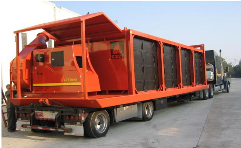
*S327 Transported on Step-deck Tractor-Trailer*
