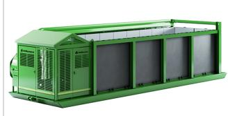
**General:** A self-contained, completely assembled above ground Air Curtain Burner (air curtain incinerator or FireBox) with a refractory lined burn-container for portable and permanent (stationary) applications. Designed for the high temperature burning of forest slash, land clearing debris, green waste, storm debris, and other waste streams in compliance with the requirements of US EPA 40CFR60.
