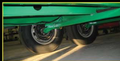
Heavy Duty Running Gear, High Ground Clearance Torsion Axles with 4- Wheel Electric Brakes
