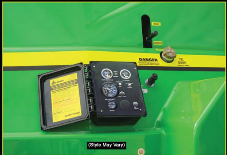
Full Engine Instrumentation with Fuel Gauge and Engine Key Switch. Locking Instrument Box, Protected Machinery and External Controls
