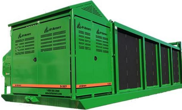
**General:** A self-contained, completely assembled above ground Air Curtain Burner (air curtain incinerator or FireBox) with a refractory lined burn-container for portable and permanent (stationary) applications. Designed for the high temperature burning of forest slash, land clearing debris, green waste, storm debris, and other waste streams in compliance with the requirements of US EPA 40CFR60.
