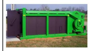
**General:** A self-contained, completely assembled above ground Air Curtain Burner (air curtain incinerator or FireBox) with a refractory lined burn-container for portable and permanent (stationary) applications. Designed for the high temperature burning of forest slash, land clearing debris, green waste, storm debris, and other waste streams in compliance with the requirements of US EPA 40CFR60.
